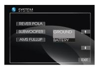
Setting REVERSE POLA in this menu. The signal is +12V when you are backing up a car, please press BATTERY in the monitor; if the signal is 0V, please press GROUND.
